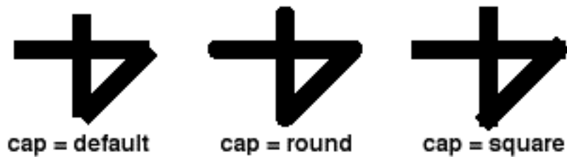
Figure 5: Example of lineMode attribute "cap"
